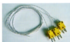
K-Type Connector with Thermocouple with Spot-Weld
